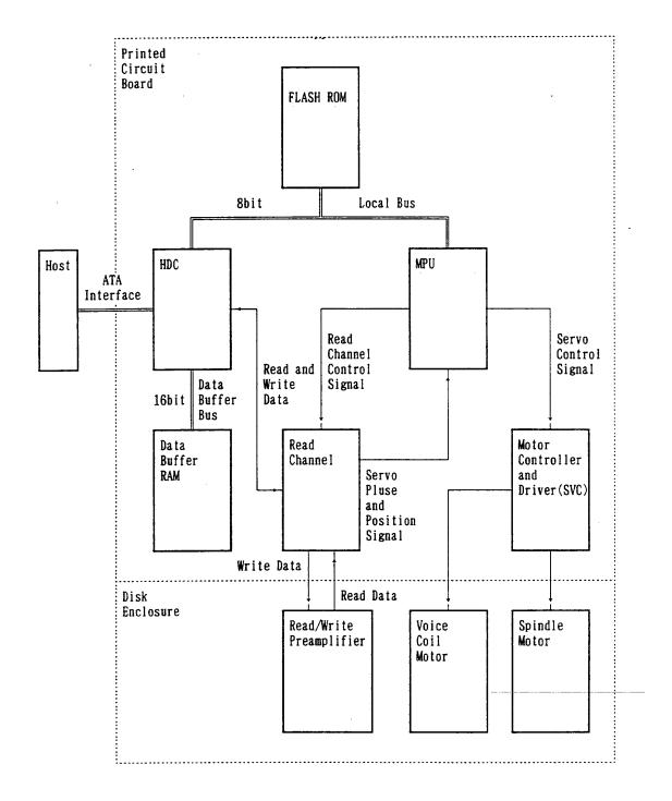
**Figure 4.2 Circuit Configuration**
